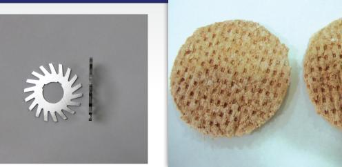
The waffle blades are wider and make a square indention on the top and bottom of the patties. These indentions create more surface area and speeds up both the freezing process and the cooking process. As shown in the picture above the indentions are retained when the patties are frozen.
