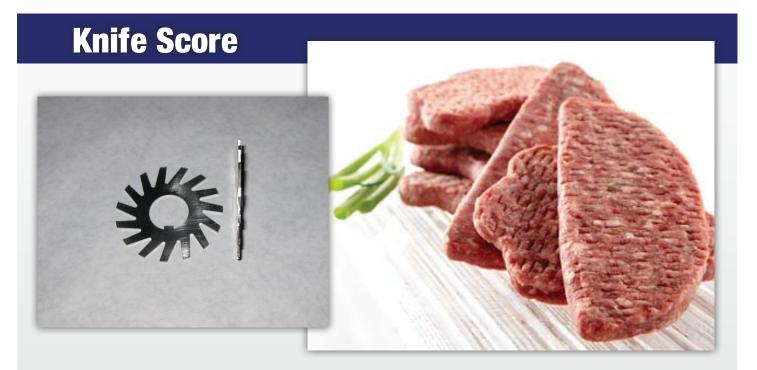
The knife blades are much thinner and come to a sharp point. These blades are offset so they can be lowered allowing the top and bottom rollers to actually mesh together. This setup allows for stretching or knitting the patties for a homemade appearance as shown in the above photo. The head can also be raised for a lighter more cosmetic appearance.
