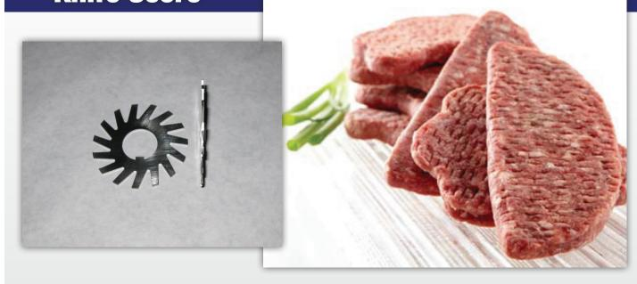
The knife blades are much thinner and come to a sharp point. These blades are offset so they can be lowered allowing the top and bottom rollers to actually mesh together. This setup allows for stretching or knitting the patties for a homemade appearance as shown in the above photo. The head can also be raised for a lighter more cosmetic appearance.
